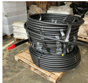
Borehole heat exchangers
